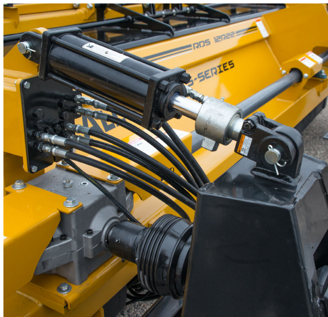
Figure 2b. PTO Driveline
