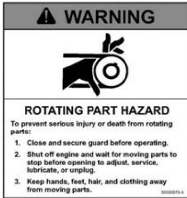
G. 500-3-0979 Rotating Part Hazard
