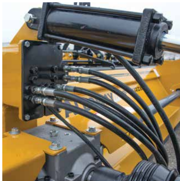
Figure 4. PTO Driveline HYDRAULIC SYSTEM
