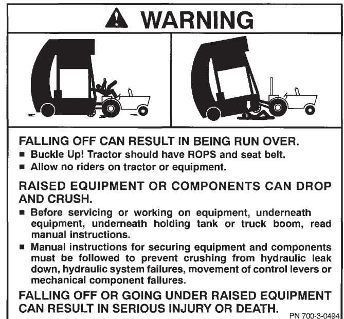
5. 700-3-0494 Fall Hazard Warning
