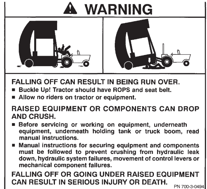
5. 700-3-0494 Fall Hazard Warning
